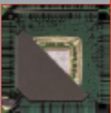
Each die is then encapsulated in a plastic molding compound, forming the 'package'. The package provides the delicate chips with physical protection and also incorporates thermal properties that enable the IC to dissipate the heat that is generated from the large number of transistors.
