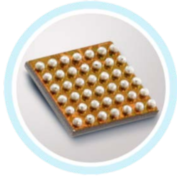
WLCSP Wafer-level Chip Scale Package (Fan-In)
