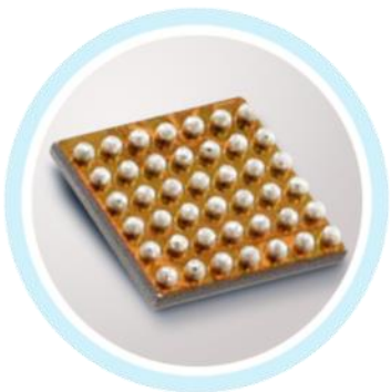
WLCSP Wafer Level Chip Scale Package (Fan-In)
